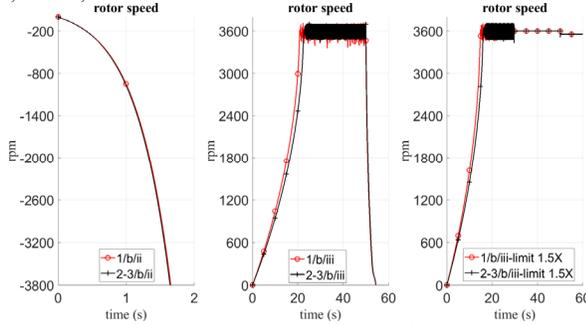
Fig. 7. Rotor speeds in configurations 1/b/ii and 2-3/b/ii (left), 1/b/iii and 2-3/b/iii (middle), and 1/b/iii and 2-3/b/iii with 1.5 times the rated current limit of the inverter (right).
