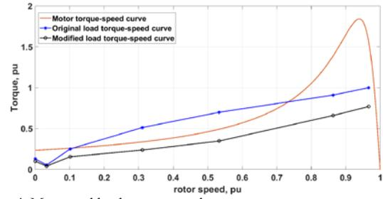
Fig. 4. Motor and load torque-speed curves.
