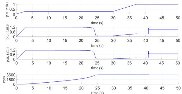
Fig. 9. Simulations results for an IBR-based motor blackstart with voltage ramp to soft start the system to suppress inrush current. Waveforms are from the top: source voltage, source current, motor current, and motor rpm.
