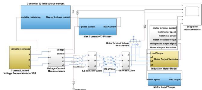
Fig. 2. Black-start simulation circuit in MATLAB Simulink/Simscape.
