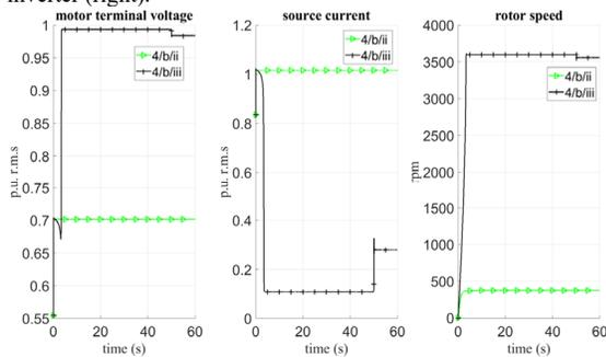
Fig. 8. Phase A voltages and currents (for one source) and rotor speeds in configurations 4/b/ii and 4/b/iii.
