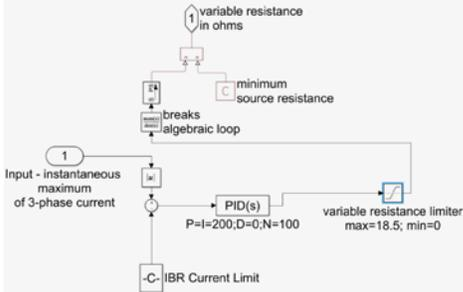
Fig. 3. Variable resistor-based inverter current limit controller.
