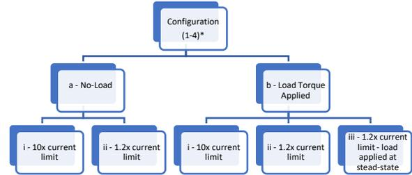
Fig. 5. Simulations run for the black-start configurations. (For configuration 4, 10-times current limit simulations were not run because one source was able to start the motor under loaded and unloaded conditions)
