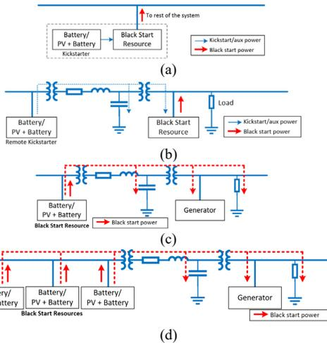
Fig. 1. Four black-start configurations for IBRs. (a)–(d) show configurations 1–4, respectively.
