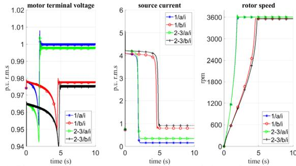
Fig. 6. Phase A voltages, currents, and rotor speeds in configurations 1/a/i, 1/b/i, 2-3/a/i, and 2-3/b/i.
