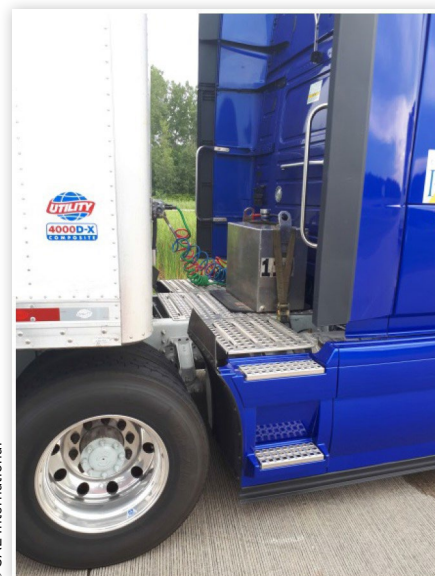
FIGURE 9 Installation of the portable fuel tanks.
