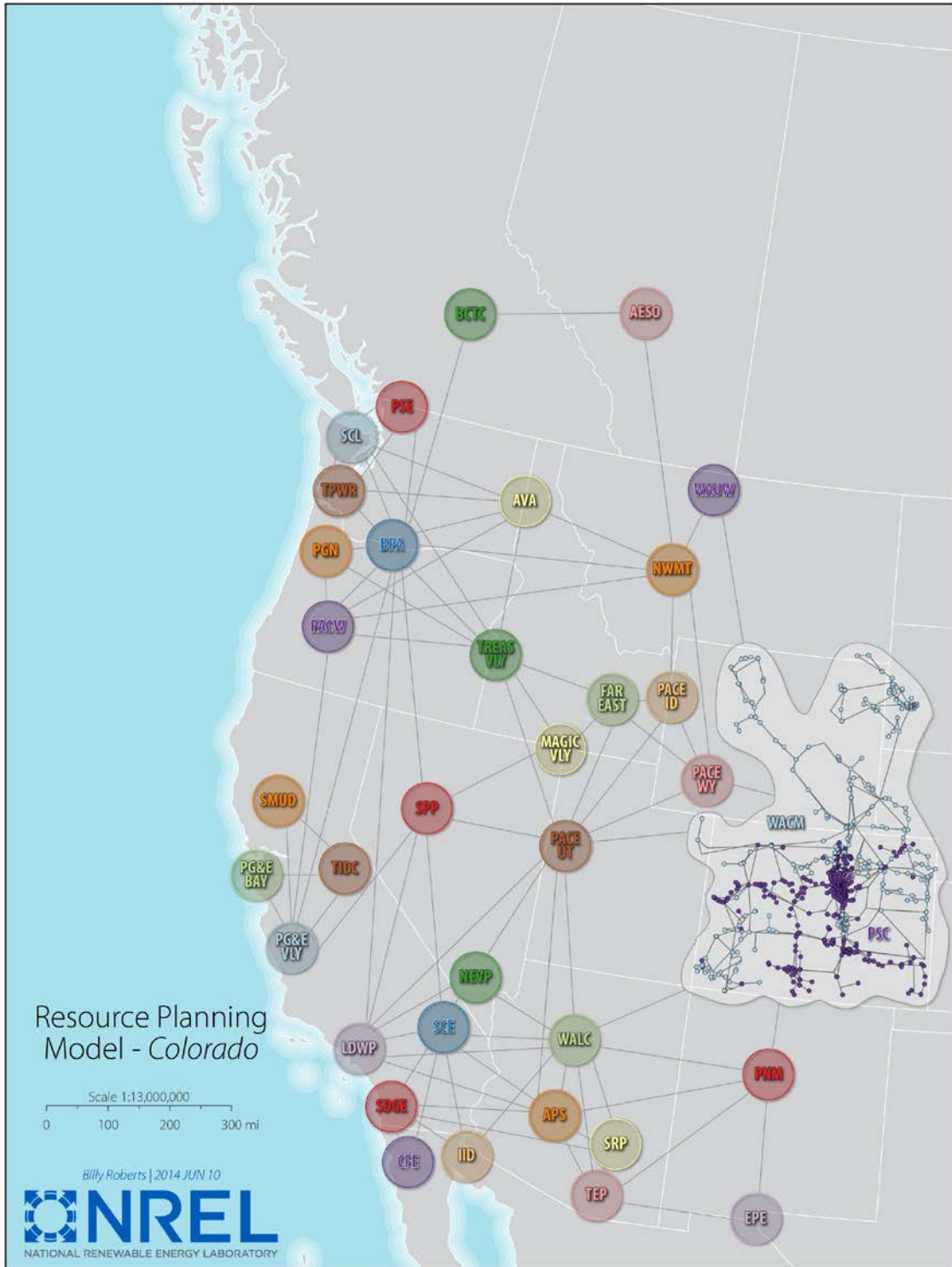
Figure 2. Combined zonal/nodal structure used for the CO-centric version of RPM
