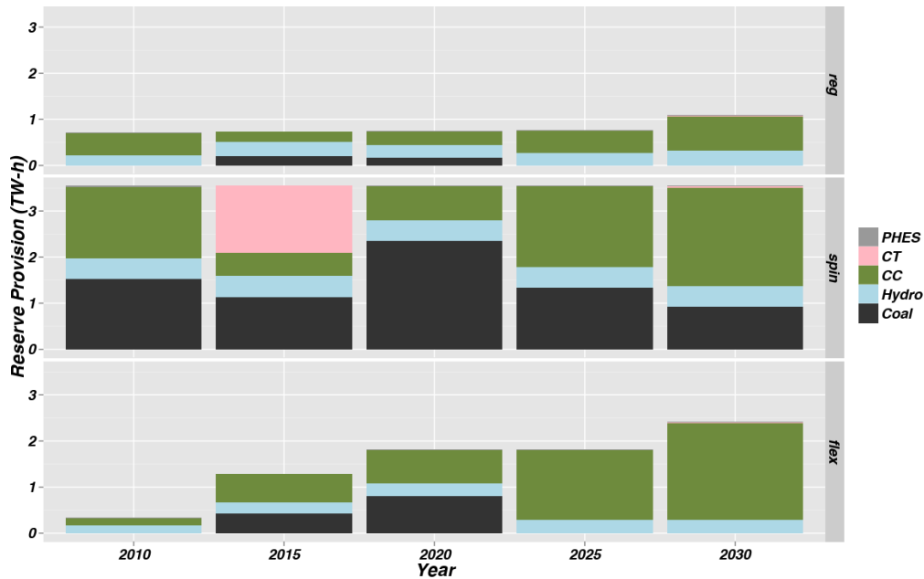
Figure 13. Annual reserve provision in the CO-centric focus region for regulation (reg), spinning (spin), and flexibility (flex) reserve products in the REF scenario
