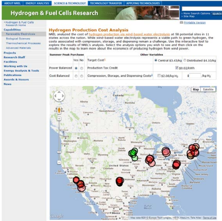
Figure 2 - Opening screen of the interactive tool, showing the entire set of analysis results, with the PTC effect turned on. Green sites meet DOE's 2015 target for centralized electrolysis ($3.10/kg)
