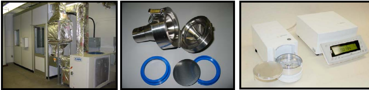
Figure A-5. Class 1000 clean room, filter housing, and microbalance
