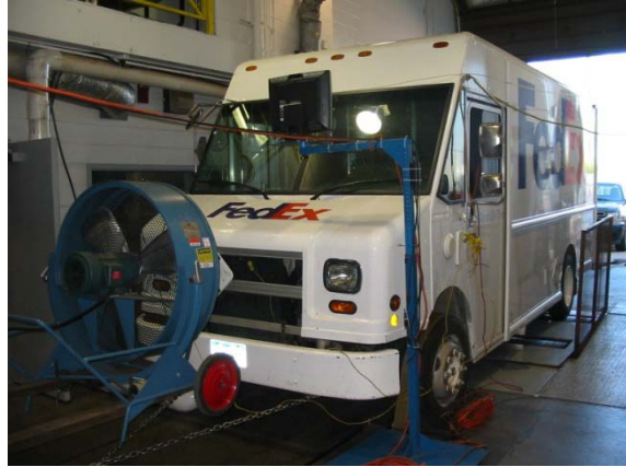
Figure A-6. Chassis cell with test vehicle
