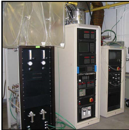
Figure A-4. Gaseous and PM sampling benches
