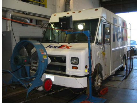
Figure A-6. Chassis cell with test vehicle
