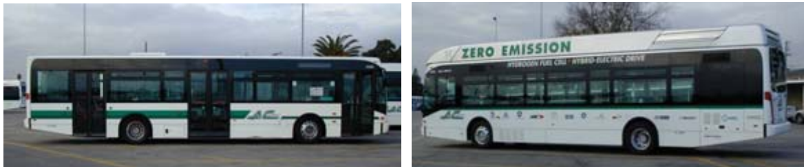
Figure ES-1. AC Transit Van Hool buses – diesel (left) and fuel cell (right)
