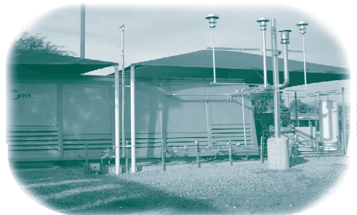
A natural gas autothermal reformer by HyRadix produces hydrogen for the fuel cell bus at SunLine.
