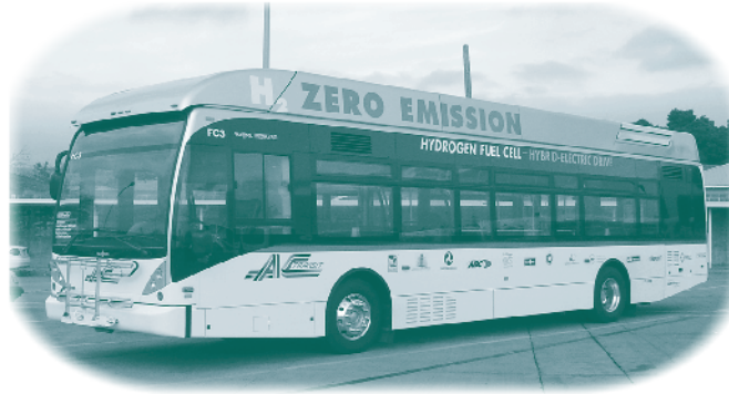
The buses at AC Transit have UTC Power fuel cell and ISE hybrid electric drive systems.
