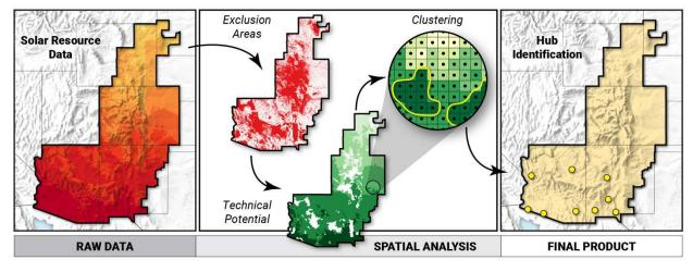
Figure 4. Workflow used by NREL to identify renewable energy zones
