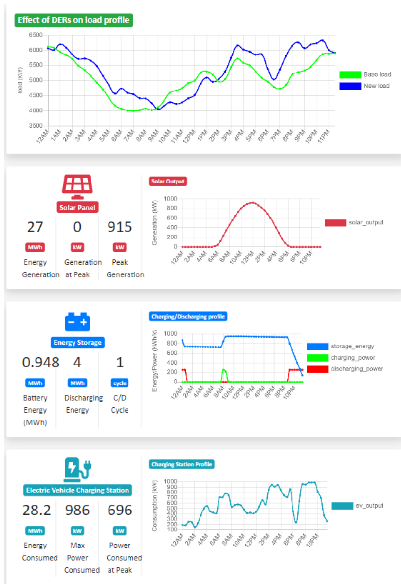
Figure 58. Impact on load profile of Feeder1 due to DERs on summer day of 2019. Starting from the top, first figure shows new and base profile, second figure shows solar generation profile (1 MW solar capacity), third figure shows battery energy, charging and discharging profile (1,000 MWh, 500 kW), and last figure shows aggregated consumption pattern of EVs (10 vehicles, 25% residential)
