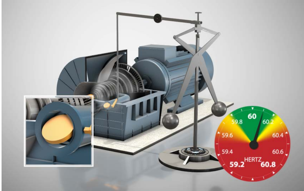
b) Frequency increases and governor closes valve, decreasing power
