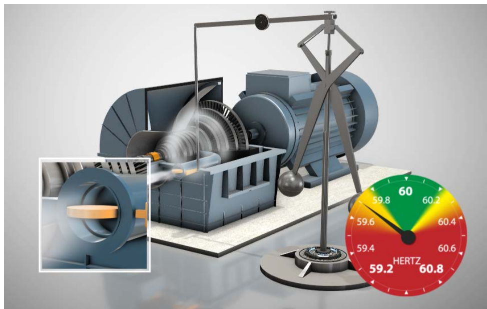
a) Frequency drops and governor opens valve, increasing power
