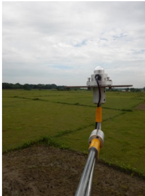
Figure 17. Insolation sensor at Mymensingh. Photo by Harness Energy.
