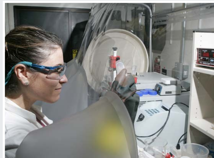
Dr. Alexandra Dubini isolates oxygen-sensitive proteins in a glove box under anaerobic conditions. Photo by Jack Dempsey, NREL/PIX 14561
