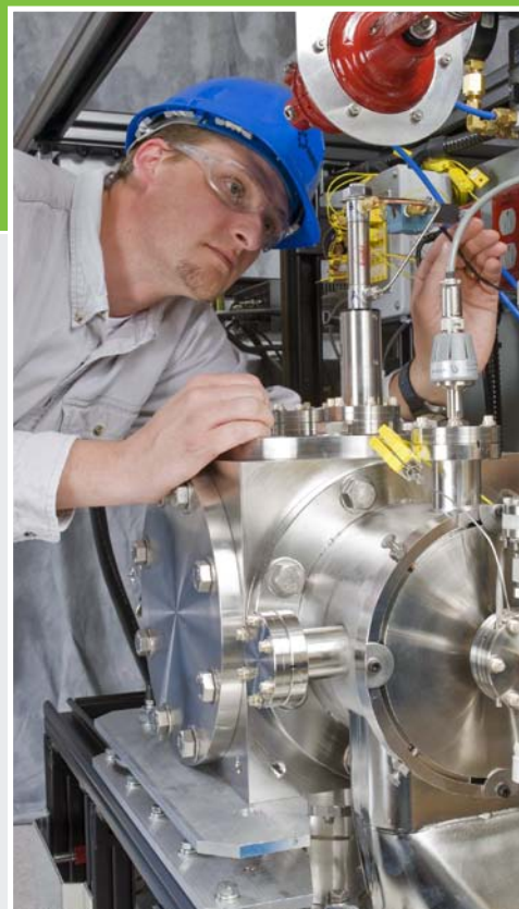
The MBMS can be used by industrial partners to analyze high-temperature vapors in thermochemical processes. Photo by Bryan Bechtold, NREL/PIX 17382
