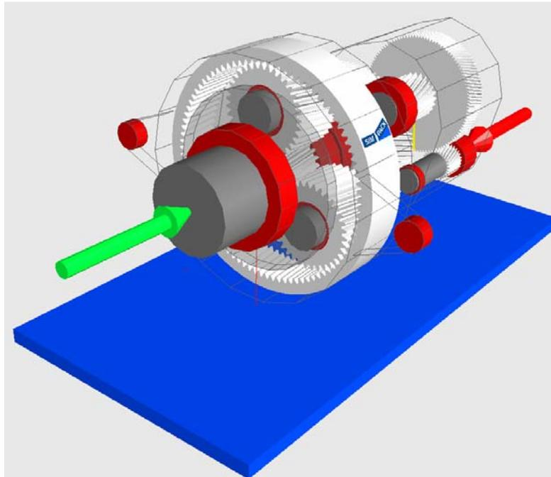
**Figure 6 - Preliminary Model of Gearbox using SimPack™ software**
