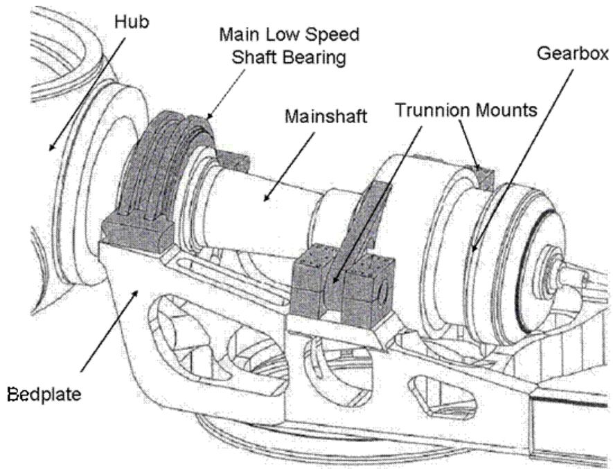
**Figure 1 – Typical Wind Turbine Gearbox Mount [10]**
