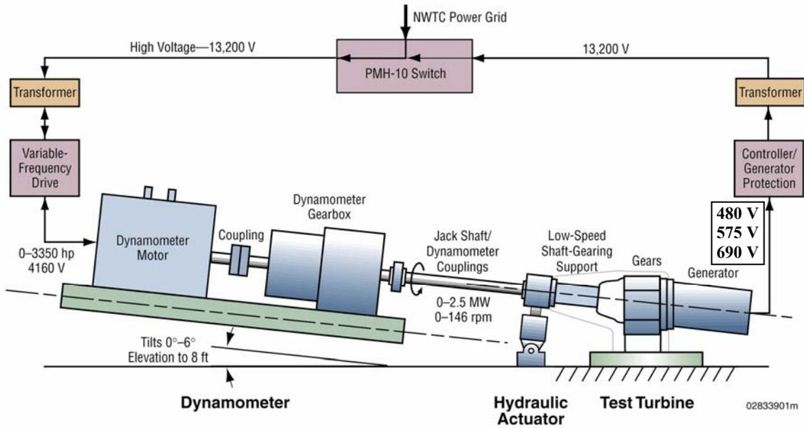
**Figure 4 – Schematic of NREL 2.5 MW Dynamometer Test Facility**
