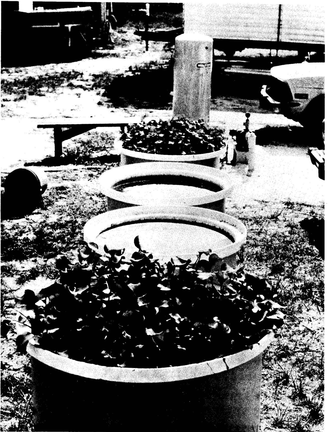
Figure 1. Cylindrical tanks used for measurement of evapotranspiration rates of freshwater macrophytes.
