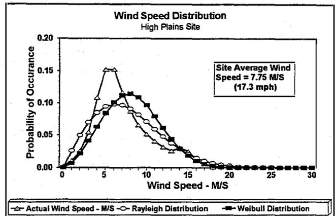
**Figure 2** WIND SPEED DISTRIBUTION AT A HIGH PLAINS SITE. RAYLEIGH C AND K ARE 8.74 AND 2.0 RESPECTIVELY, AND THE WEIBULL C AND K ARE 9.31 AND 2.66 RESPECTIVELY.
