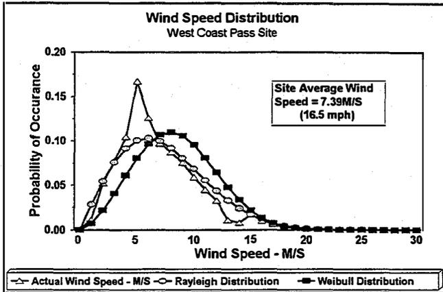
**Figure 1** WIND SPEED DISTRIBUTION AT A WEST COAST PASS SITE. RAYLEIGH C AND K ARE 8.34 AND 2.0 RESPECTIVELY, AND THE WEIBULL C AND K ARE 9.53 AND 2.61 RESPECTIVELY.
