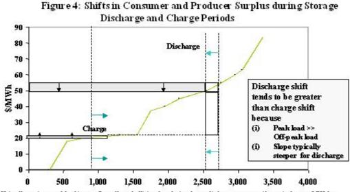
Note: Charge increased by  $l/\eta$  to reflect effect of efficient loss during charge discharge process – Alternatively same MW for charging and discharging but  $l/\eta$  times the discharge period
