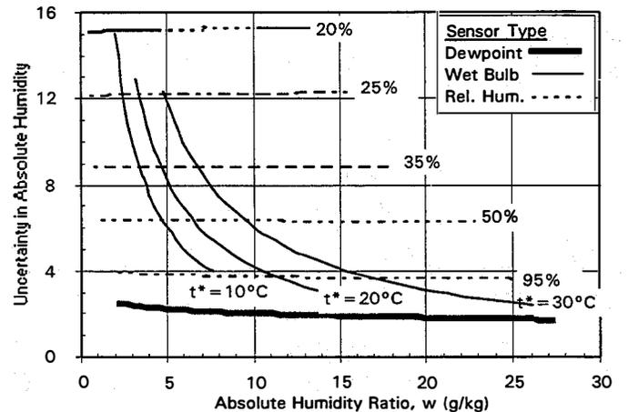
**Figure 1. Uncertainty Analysis Results Using "Standard Accuracy" Instrumentation**
