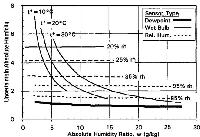
Figure 4. Uncertainty Analysis Results Using "High Accuracy" Instrumentation
