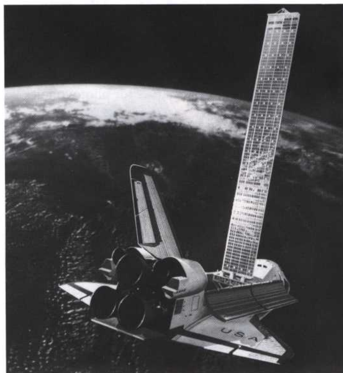
Photovoltaic cells were first used in space to power a 5-mW backup transmitter on the Vanguard 1 in 1958. Today, solar cells power most satellites; even the U.S. shuttle fleet uses PV to generate much of its electrical power. (Rendition courtesy of Lockheed.)
