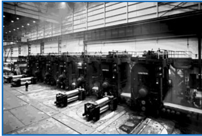
This hot strip mill is the largest electrical-power consumer at Burns Harbor, with about half of the energy going to power pumps and fans.
