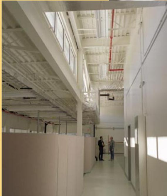
The Thermal Test Facility at NREL in Golden, Colorado, incorporates daylighting, passive solar heating, ventilation, evaporative cooling, high performance lighting, and mechanical systems into its design. The building is expected to use at least 70% less energy than one meeting existing energy standards and to save 65% in HVAC energy costs.
