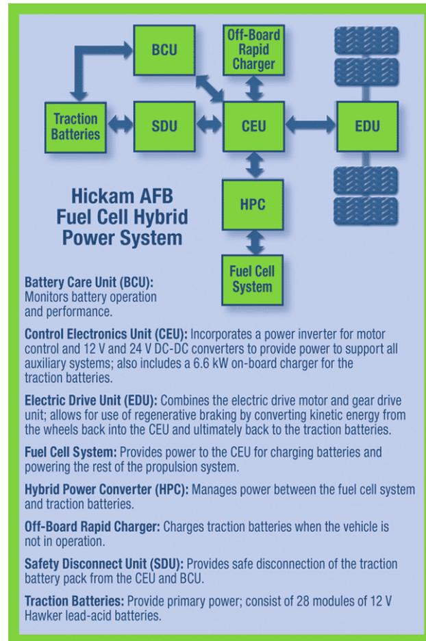
**Figure 3.** Hickam Air Force Base Fuel Cell Hybrid Power System
