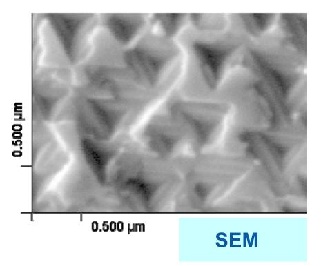
Cu-Mediated Surface Morphology of CdTe(111)-B
