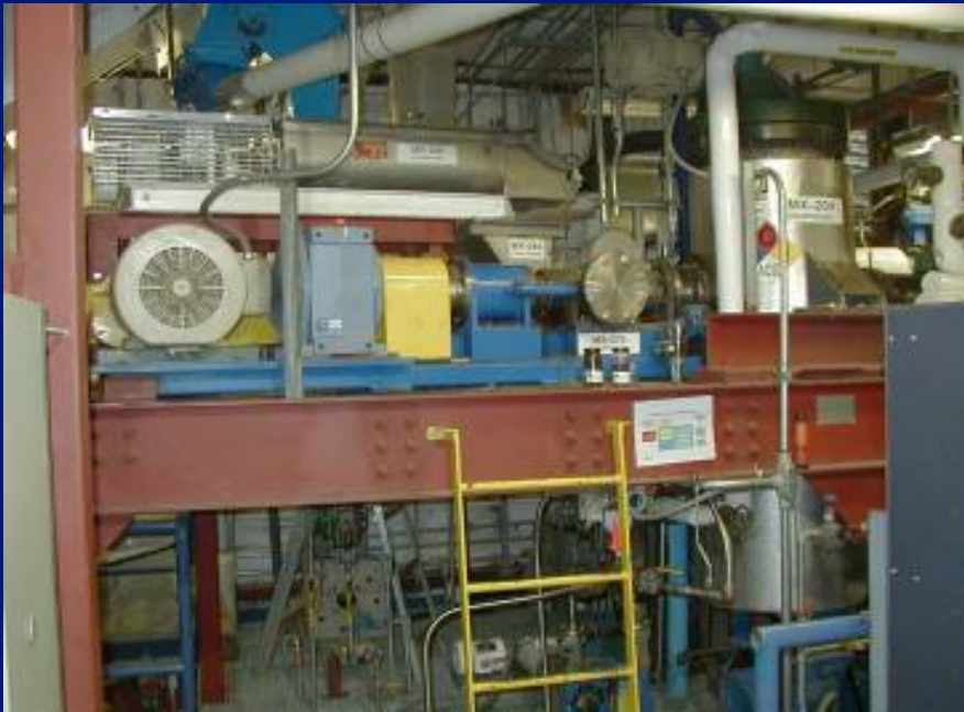
1 ton/day Sands Continuous Pretreatment Reactor
