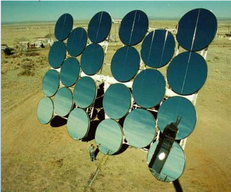
Heliostat at the National Solar Thermal Test Facility (Sandia)
