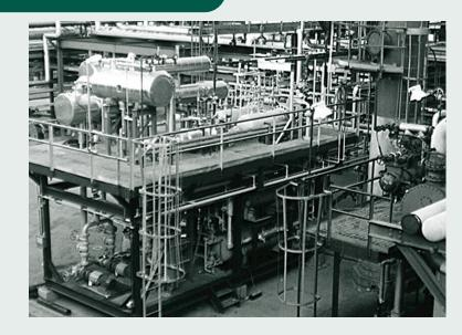
A prototype of the critical components for the absorption system. Data from the prototype indicate that the Industrial Refrigeration System (critical components pictured above) could cut fuel consumption by 19 trillion Btu and cut greenhouse gas emissions by more than 1 million tons per year.
