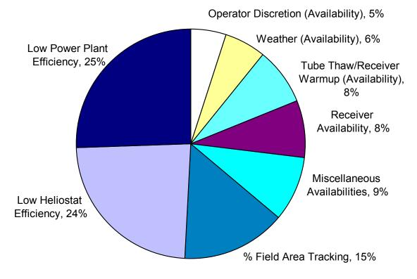
Figure 6: September 1998 Solar Two Gross Electricity Loss Contributions
