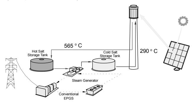
Figure 1: Schematic of a Molten-Salt Central-Receiver Power Plant
