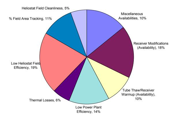
Figure 7: October 1998 Solar Two Gross Electricity Loss Contributions
