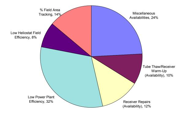
Figure 4: June 1998 Solar Two Gross Electricity Loss Contributions
