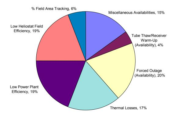
Figure 5: July 1998 Solar Two Gross Electricity Loss Contributions
