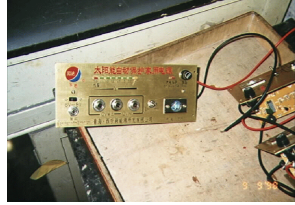
2. Xining - Typical SHS Controller Panel
