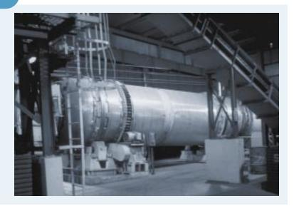
Indirect-fired IDEX kilns are demonstrating how secondary aluminum smelters can obtain higher-quality feedstock from metal scrap without emitting pollutants during the decoating process.
