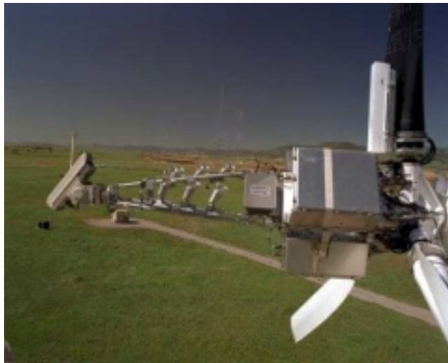
Figure A.2. Hub-mounted instrumentation boxes, boom, and camera.
