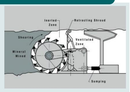
This illustration of the Variable Wall Mining Machine shows the variable cutting heads equipped with helical vanes to move the cut coal through the center of the machine toward stage loaders.
