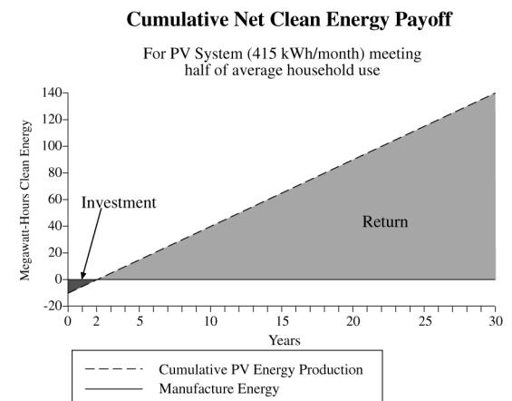
PV systems can repay their energy investment in about 2 years. During its 28 remaining years of assumed operation, a PV system that meets half of an average household's electrical use would eliminate half a ton of sulfur dioxide and one-third of a ton of nitrogen oxides pollution. The carbon dioxide emissions avoided would offset the operation of two cars for those 28 years.
