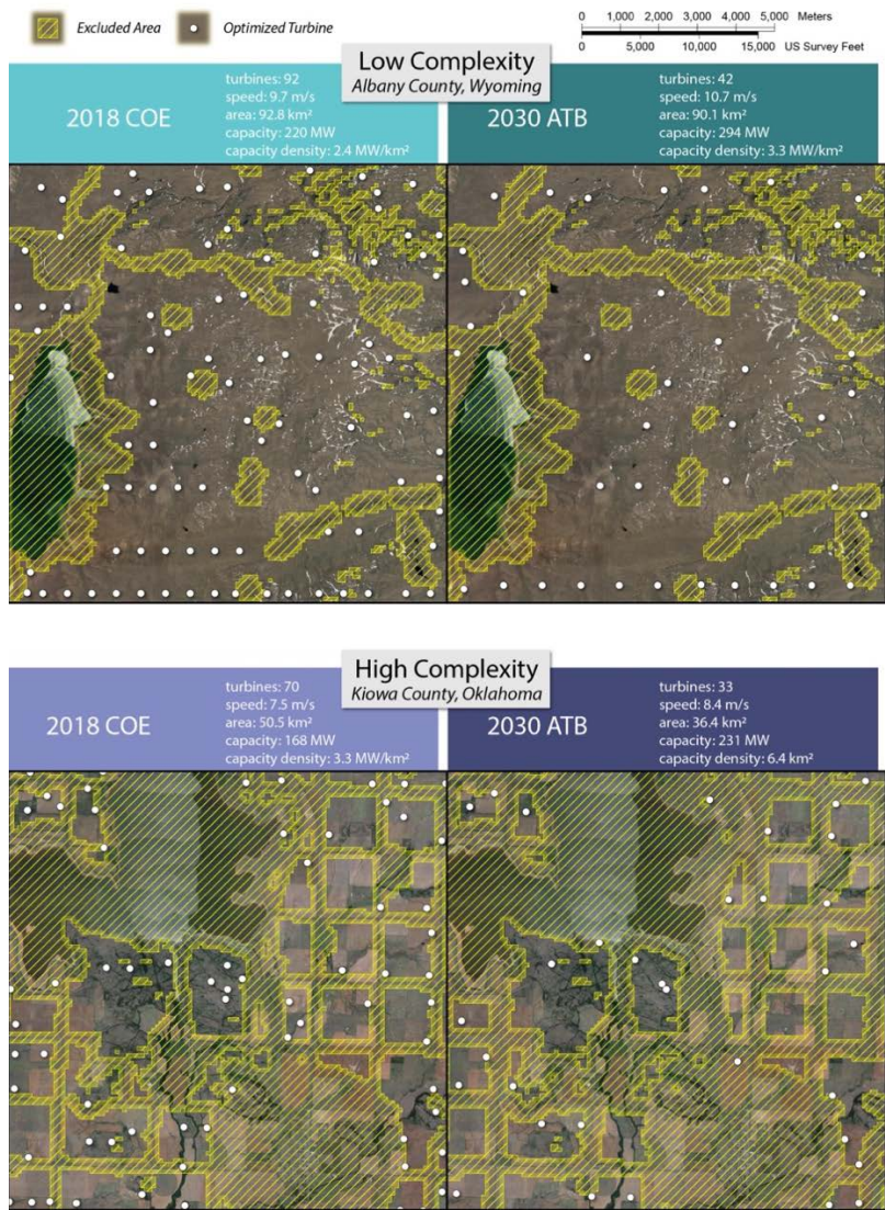
Figure 3. Cross section of wind site drivers showing a low complexity site and a high complexity site with different turbine assumptions. It may appear some turbines violate the spatial constraints; however, this is simply due to the scale of the image.
