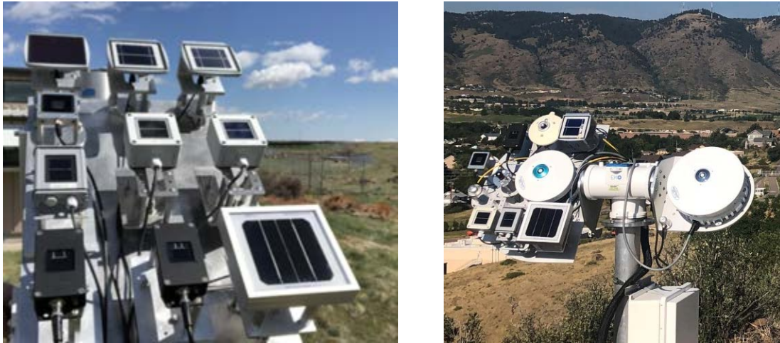
Figure 1. Reference cells installed for field observations at the SRRL. Photos by NREL
