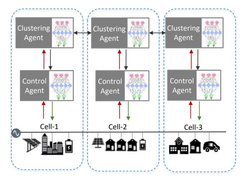
Use **Multi-Agent Deep Reinforcement** Learning (MADRL) to design a 2-Level Control Strategy for managing DERs in coordination with network reconfiguration for both normal grid-connected and resilient microgrid operations:
