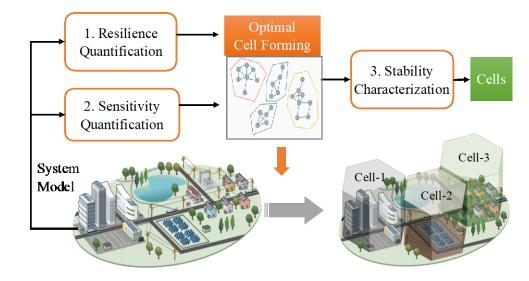
Each identified cell has integrated resilience over a desired threshold and can achieve stable operation when disconnected from the grid.
