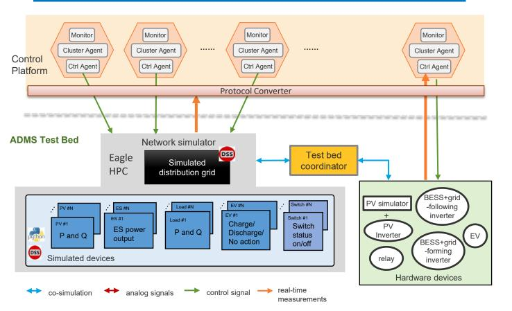
A distributed ADMS solution with extensive DER control capability
