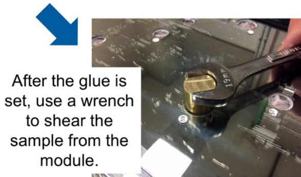
Figure 9. Coring procedure to extract defect-containing samples from a module.
