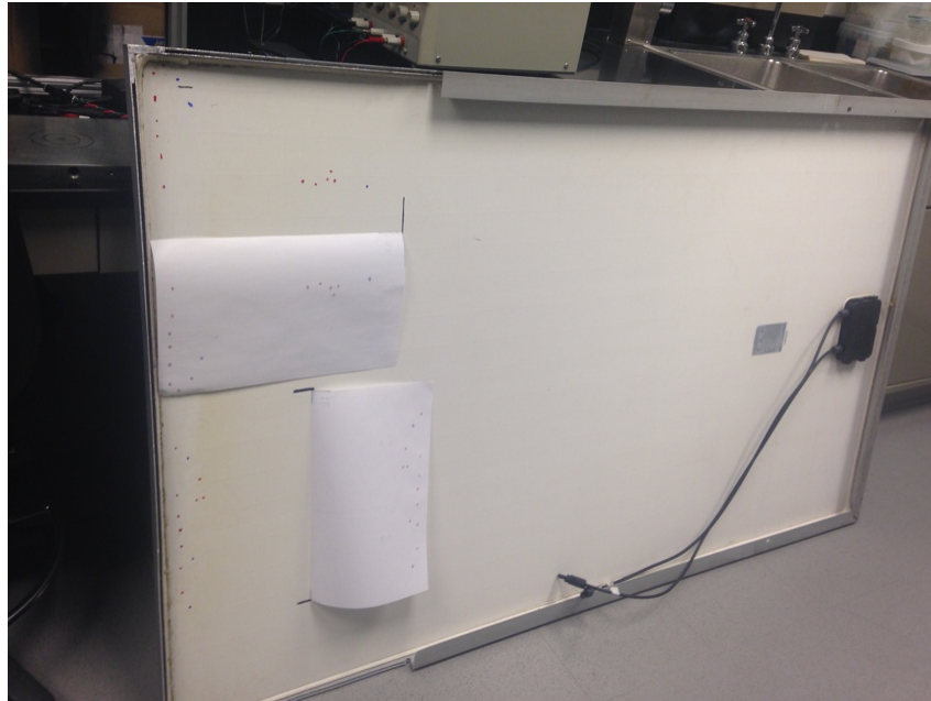
Figure 5. Regions of interest for coring are marked directly on the backsheet of a silicon module. Paper duplicate maps are taped in place so that the regions can be accurately relocated after removing the backsheet in the coring locations.
