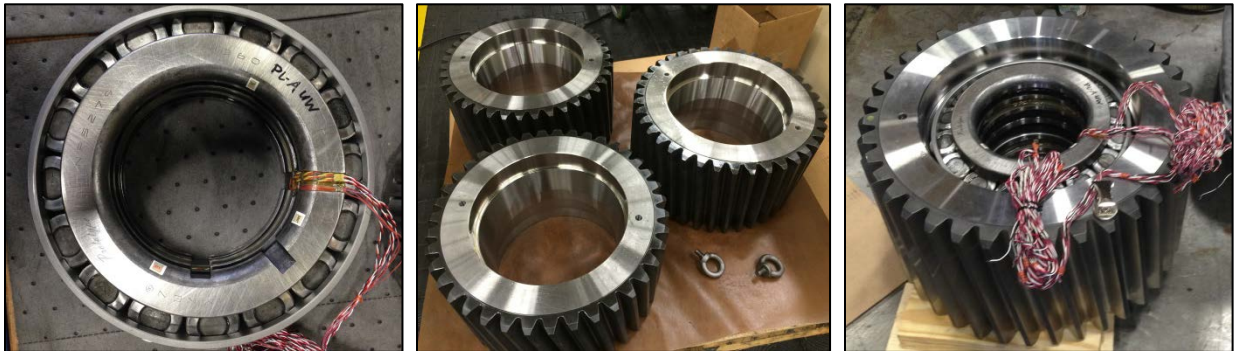
Figure 5. Planet bearings and gears. Photos by Jonathan Keller, NREL 36523, 36524, and 36520
