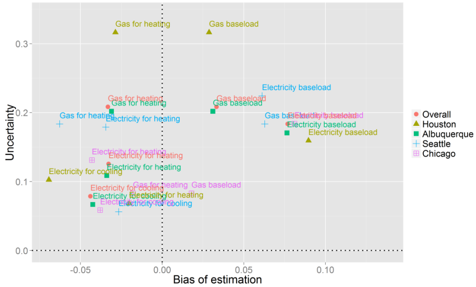
Figure F-24. Bias and uncertainty of energy end use ratio estimates for medium office buildings under different climate zones
