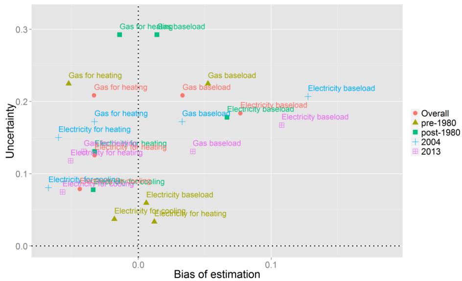
Figure F-23. Bias and uncertainty of energy end use ratio estimates for medium office buildings under different vintages
