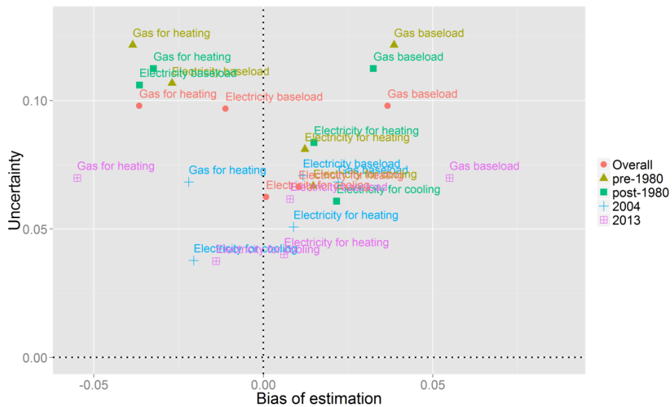
Figure F-25. Bias and uncertainty of energy end use ratio estimates for standalone retail buildings under different vintages
