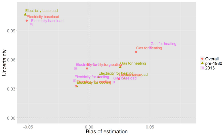
Figure F-39. Bias and uncertainty of cost ratio estimates for main-street buildings under different vintages
