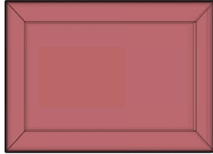
Figure A-2. Division of thermal zones for the medium office model (Thornton et al. 2011)
