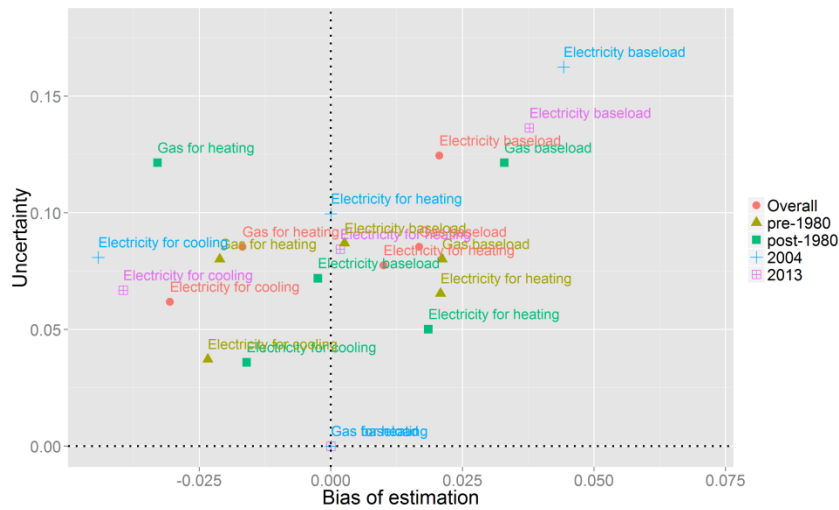
Figure F-21. Bias and uncertainty of energy end use ratio estimates for small office buildings under different vintages
