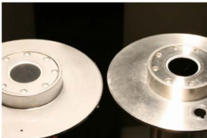
Damaged NIP side by side with undamaged NIP. Also note that the mirrored chrome surface has been dulled to a matte surface.
