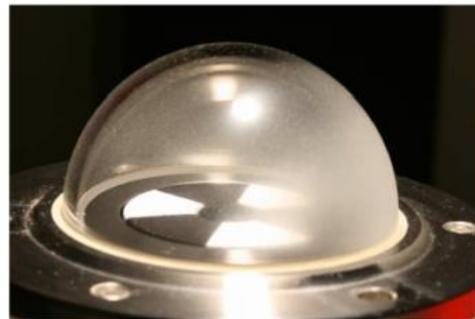
8-48. Note directional effect of damage (greatest effect is near the connector)
