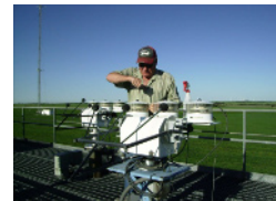
Figure 6. Craig Webb installing pyrgometers on one of the LW trackers at the SGP RCF.
