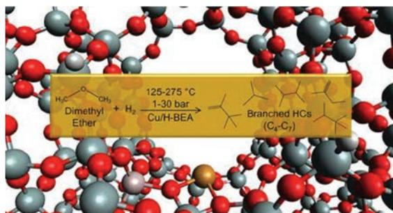
Recent research shows that the addition of a newly formulated copper catalyst allows more hydrogen to be incorporated into the biomass-to-liquid-fuel process, thus increasing production rates and decreasing unwanted byproducts. Image by Carrie Farberow and Joshua Schaidle, NREL.
