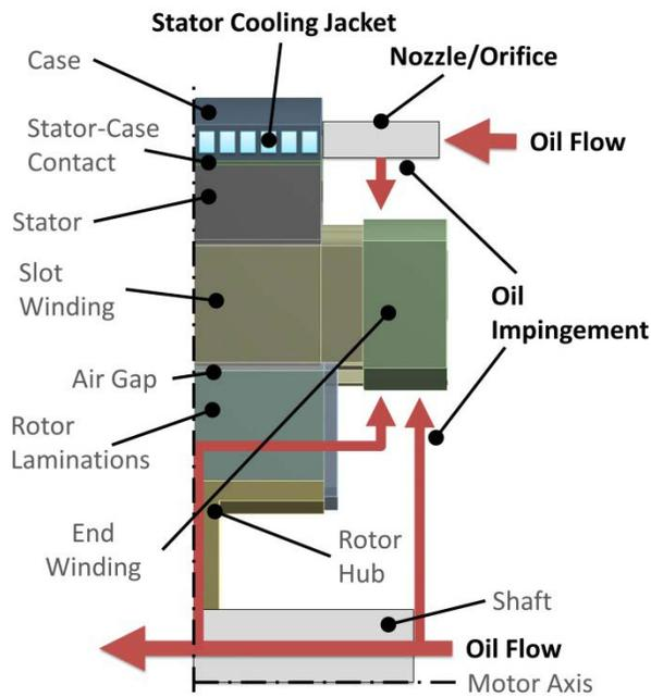
Figure I-2: Heat must pass through several layers within the motor to be extracted through active cooling such as through a cooling jacket or spray cooling with oil such as ATF.
