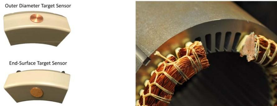
**Figure I-12: Assembled sensor packages for outer diameter surface measurement and end surface measurement (left), stator winding removed for sensor package (right)**
