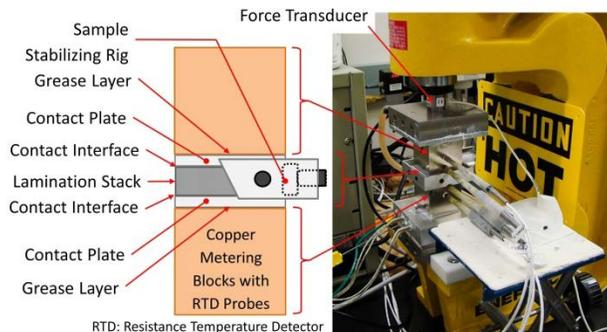
**Figure I-16: Experimental setup for measuring stator-to-case thermal contact resistance and lamination in-plane thermal conductivity under high pressure**
