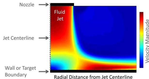
Figure I-4: Experimental velocity profile of jet impingement showing variation in velocity at the target or wall boundary. Data measured using particle image velocimetry equipment at NREL.
