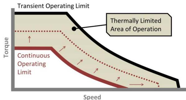
**Figure I-1: Thermal management impact on motor performance to support increased power**
