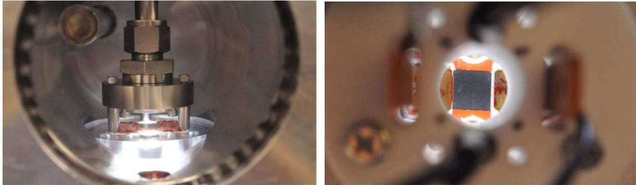
**Figure I-9: Test article and nozzle assembly (left), assembled test article showing camera view of illuminated TLC surface (right)**
