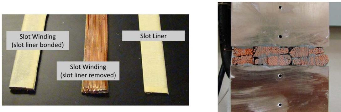
**Figure I-14: Images of sample slot-winding materials (left), sample slot winding under test for measuring cross-slot thermal conductivity (right)**
