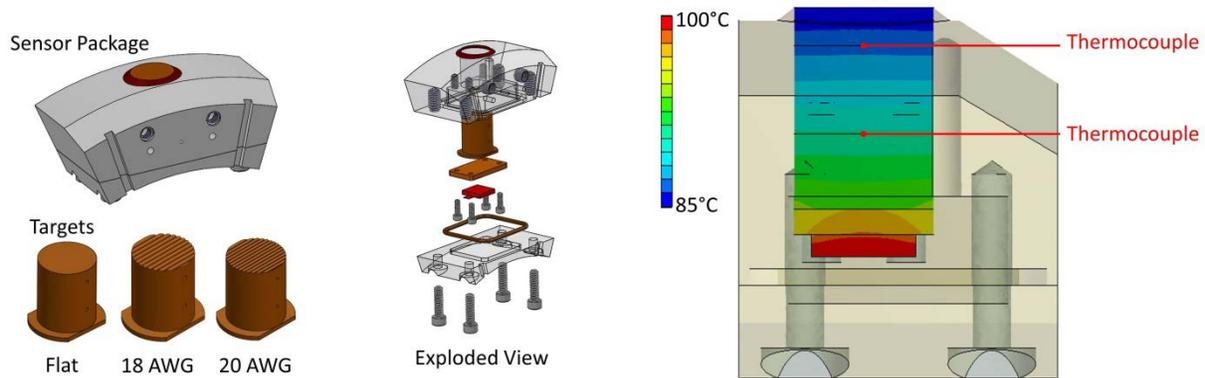
**Figure I-11: Design of sensor package showing assembled components and ability to change target surfaces (left), thermal finite element model of sensor package design (right).**
