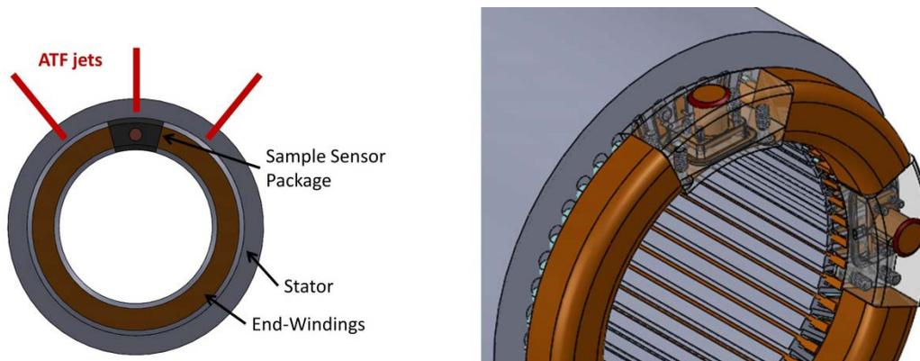
**Figure I-10: Illustration of sensor package installed in end winding (left), three-dimensional drawing of stator end winding with sensor package installed for convective heat transfer measurements (right)**
