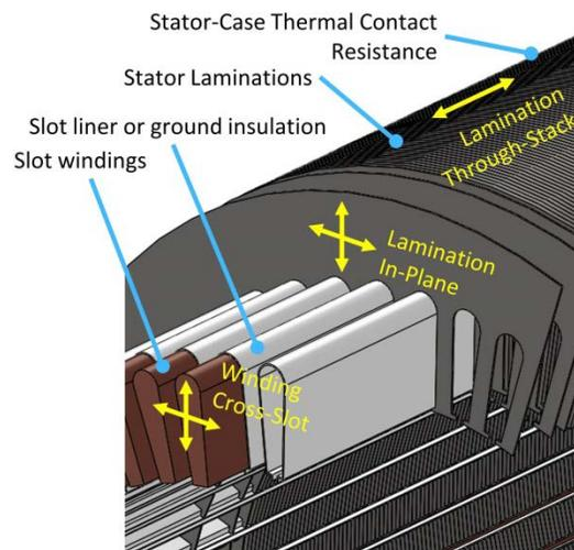
Figure I-6: Passive stack thermal properties and terminology.
