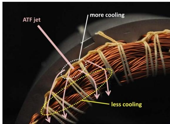
Figure I-5: Heat transfer due to ATF jet impingement will vary over the end-winding surface.
