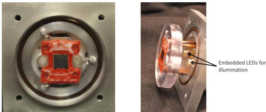
**Figure I-8: Assembled test article showing impingement surface (left), Assembled test article showing embedded LEDs to illuminate the TLC surface (right).**
