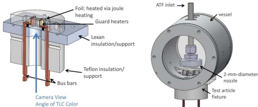
**Figure I-7: Cross-sectional view of TLC test article (left). Test article with nozzle assembly (right).**
