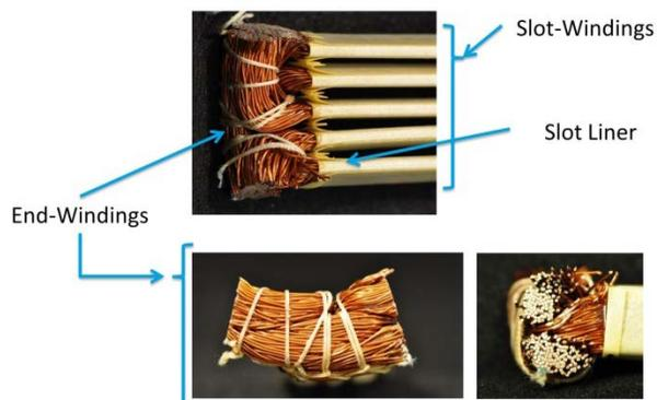
**Figure I-13: Images of sample slot-winding and end-winding motor components**
