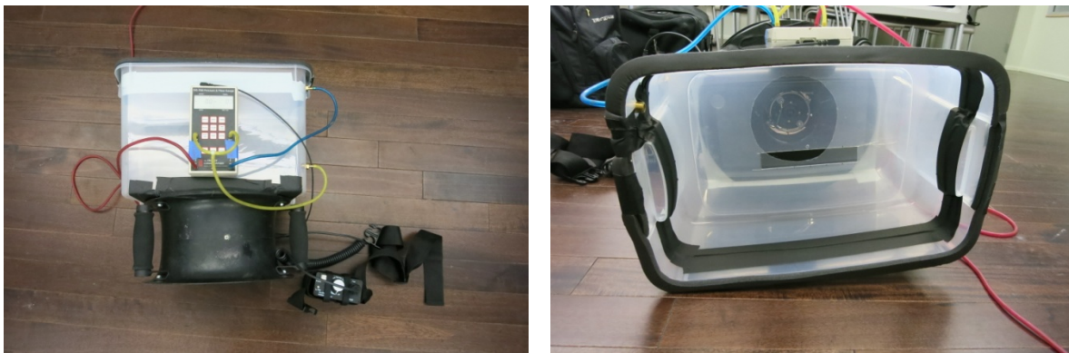
Figure 19. Setup for testing airflow through airlets
