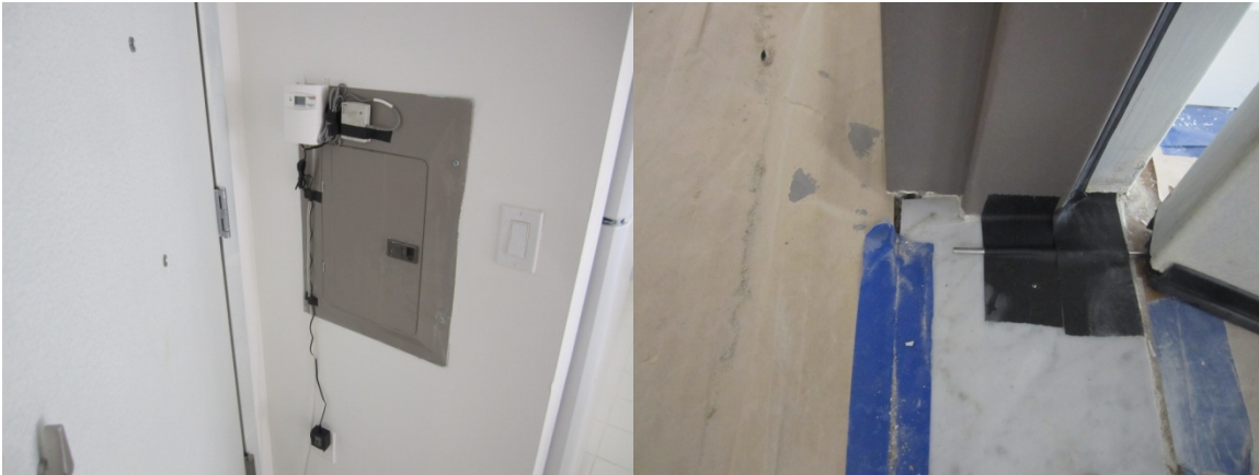
Figure 8. Placement of pressure transducer under corridor door
