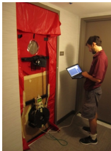
Figure 32. Setup for testing airflow around door with a blower door shroud and Duct Blaster fan
