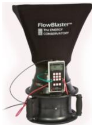
Figure 4. Powered flow hood. Image from The Energy Conservatory
