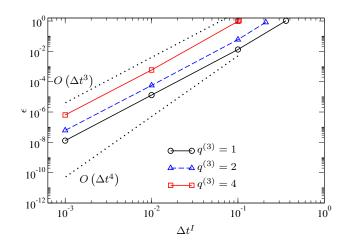
Figure 13. Normalized RMS error of  $u^{(1)}(t)$  displacement histories for Partition 1 coupled to Partition 3 for  $0 \le t \le 100$ . Partitions 1 and 3 were both time integrated with ABM4;  $\Delta t^{(1)} = \Delta t^I$  and  $\Delta t^{(3)} = q^{(3)} \Delta t^I$ . Dotted lines show ideal third-order and fourth-order convergence rates.
