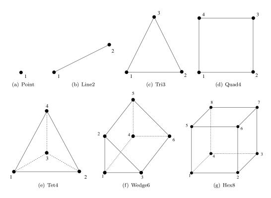
Figure 3. Interface-element types in the modularized FAST framework for coupling partitions.
