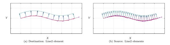
Figure 6. Demonstration of the Line2\_to\_Line2 mapping algorithm: Load mapping. (b) Nodes of Source Line2 elements show values of distributed forces (turquoise vectors). (a) Destination Line2 distributed forces after mapping. Also shown are the orientations (orthogonal pairs of purple vectors) from Figure 5.
