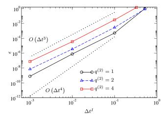
Figure 10. Normalized RMS error of  $d^{(1)}(t)$  displacement histories for Partition 1 coupled to Partition 2 for  $0 \le t \le 50$ . Partitions 1 and 2 were both time integrated with ABM4;  $\Delta t^{(1)} = \Delta t^I$  and  $\Delta t^{(2)} = q^{(2)} \Delta t^I$ . Dotted lines show ideal third-order and fourth-order convergence rates.
