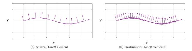
Figure 5. Demonstration of the Line2\_to\_Line2 mapping algorithm: Motion mapping. (a) The source Line2 elements are "flattened" in the positive X-direction as shown. (b) Destination Line2 elements after motions have been mapped. Orientations are shown as orthogonal pairs of purple vectors.
