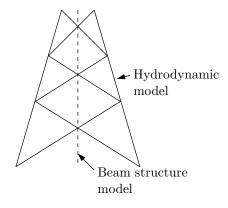
Figure 2. A multi-member hydrodynamics partition overlayed on a single-beam structural partition.
