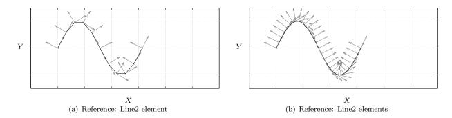
Figure 4. Demonstration of the Line2\_to\_Line2 mapping algorithm: Reference positions and orientations. (a) Reference position and orientation of 10 Line2 interface elements, which have motion output and force/moment input. (b) Reference positions and orientations of nodes along an assembly of 30 Line2 interface elements, which have motion inputs and force/moment outputs. The grey arrows are shown as orthogonal pairs illustrating orientations defined by a DCM at each node.
