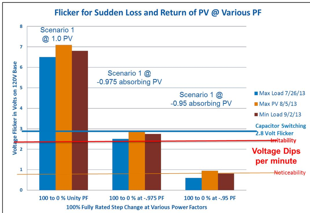
**Figure 3.15. Porterville example study results—flicker associated with sudden loss and return of rated PV at the POI compared to the fixed absorbing power factor**
