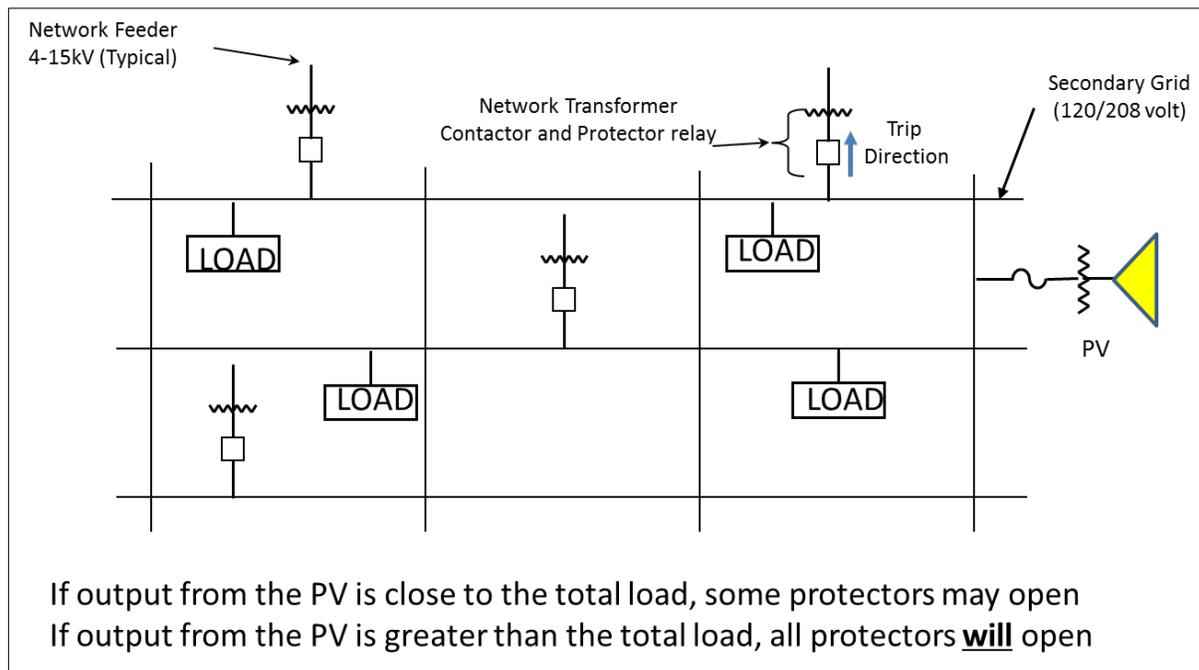
Figure 2.16. Reverse power relay operation because of PV
