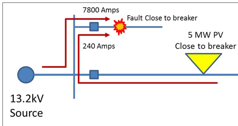
**Figure 2.9. Impact of PV on breaker interruption ratings**
