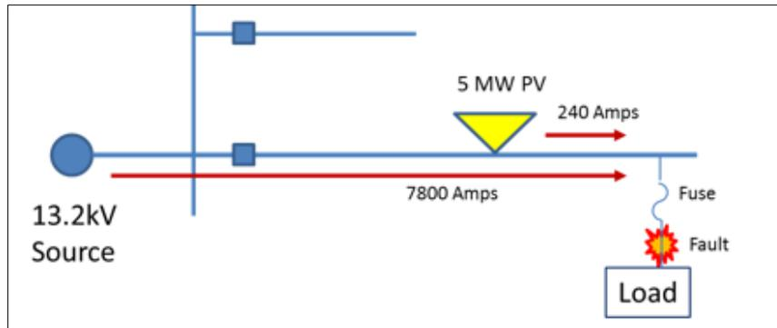
**Figure 2.8. Impact of PV on fuse interruption ratings**
