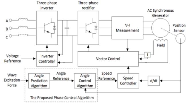
Fig. 7. Control schematics of the machine drive system
