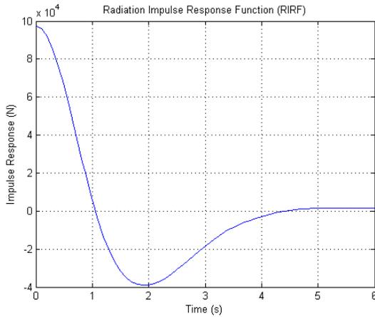
Fig. 1. Radiation impulse response function of the buoy
