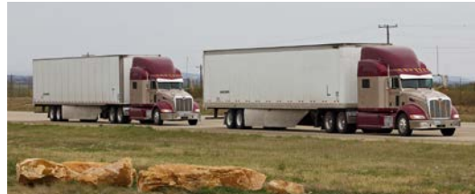
NREL conducted track testing of platooned trucks with 53-ft trailers at the 8.5-mile Uvalde track in San Antonio, Texas.
