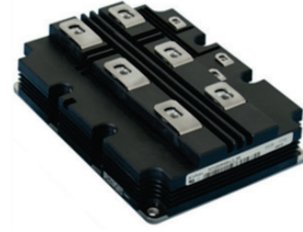
Fig. 6(a). “Fluted” 10.4-kV isolated IGBT/SiC hybrid module [19].
