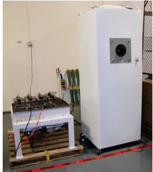
Fig. 5(a). Completed single phase test fixture as described in Fig. 2(b).
